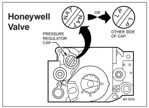
Figure 23. Convertible Pressure Regulator Cap
